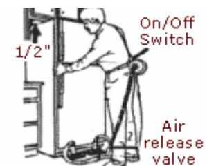
turning it off and on to provide enough air for movement without a high forceful lift. Test these methods carefully to ensure you will have enough clearance. If you have extremely low overhead clearance, an Airsled ball valve accessory may be needed.
